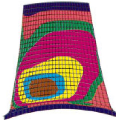
Stress distribution at 3600 rpm
