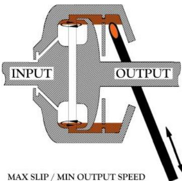
One is a straight tube with a scoop shaped tip that goes directly in and out and is mounted on an angle of roughly 20 degrees. Sketch of assembly from top.
