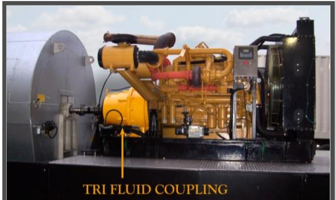
**Fluid Couplings** rated 600 hp to 1200 hp for use with Diesel engines.
