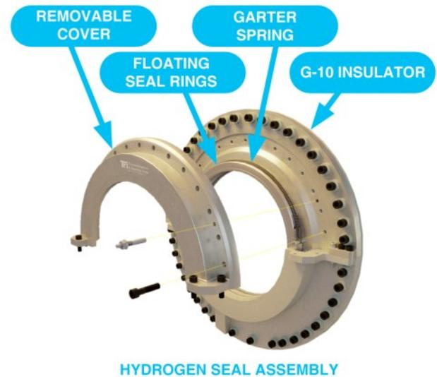
**A critically important feature of the TRI hydrogen seal design is that the housing has a removable outer top half that permits much easier installation, removal, and maintenance of the seal rings and associated garter springs.**
