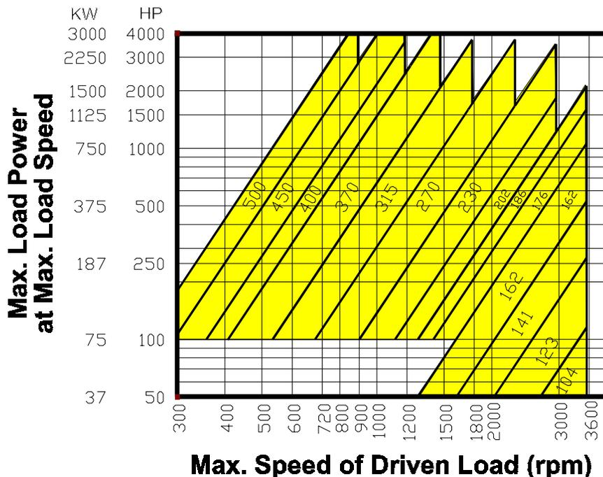
**Example:** A fan is to be driven initially at 900 hp and 1400 rpm. After an expansion of the plant, the fans normal operating point will be 1600 hp and 1700 rpm. Select a standard size 315 fluid drive and a standard size induction motor: 1750 HP, 1800 rpm.
