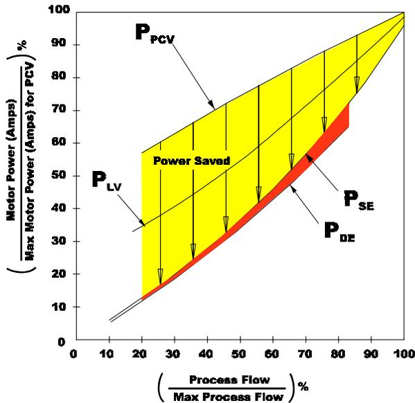
$P_{PCV}$ : Electric power to a motor, flow controlled by a discharge flow control valve
